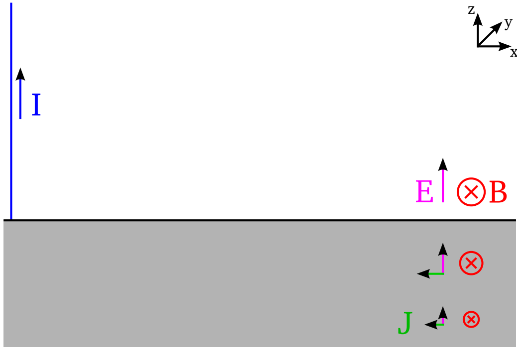
Figure 2.3.1: A Cartesian representation of the problem described in Figure 2.0.1. The vertical lightning channel to ground is far off in the -\hat{x} direction. This means that there is a magnetic field in the +\hat{y} direction and an electric field in the +\hat{z} direction above the conductor. Inside the conductor, the spatial gradient of the magnetic field will induce a current density in the -\hat{x} direction.
